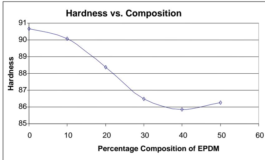
Figure 7: Hardness at Different Composition of Recycled EPDM
