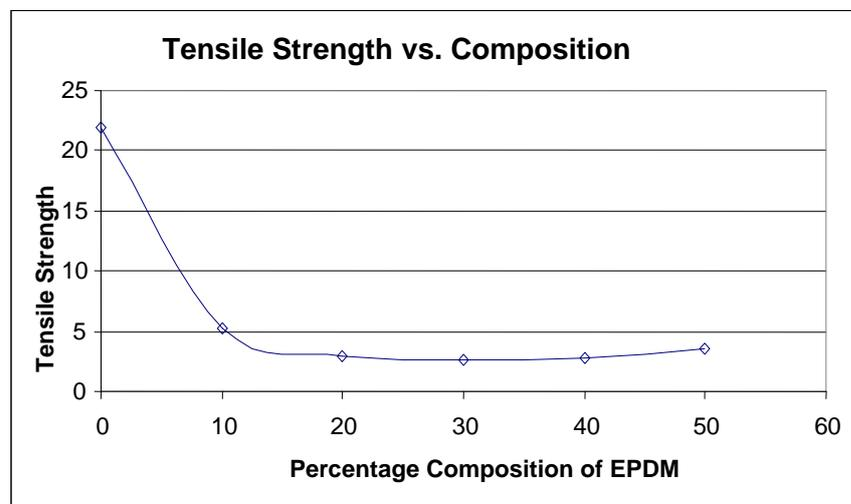
Figure 6: Tensile Strength at Different Composition of Recycled EPDM
