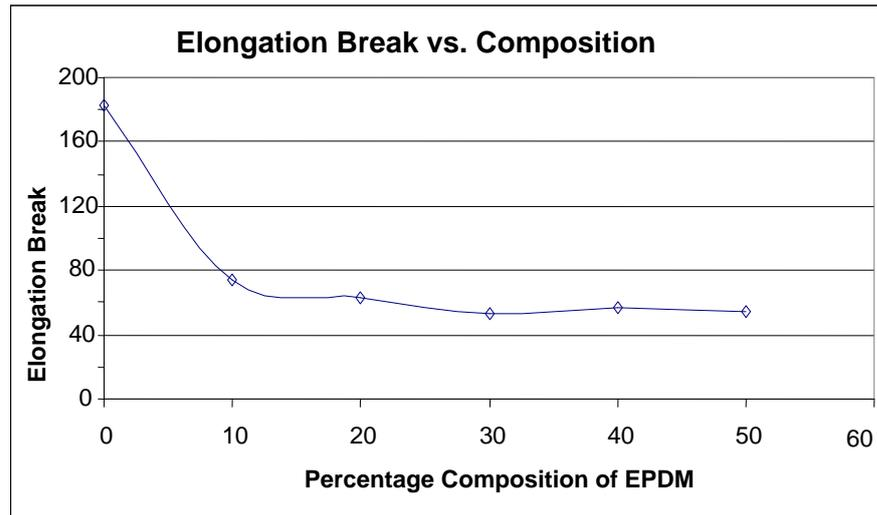
Figure 5: Elongation Break at Different Composition of Recycled EPDM
