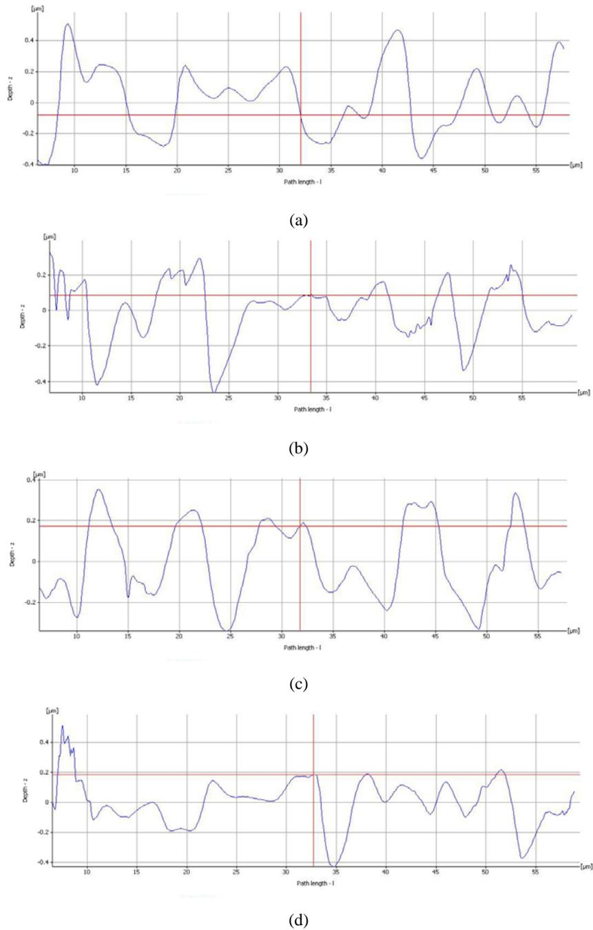
Figure 6. Shows the comparison of  $R_a$  values that represents various average roughness profile for the texture on underside of the bonded ball over the evaluation length for sample of run 3.
