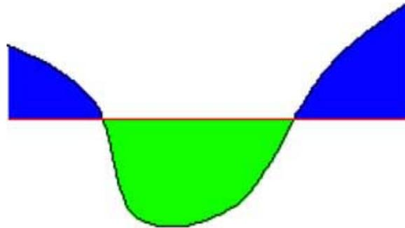
Figure 3. Volume above (blue) and below (green) the cutting plane represent the calculated volumes.
