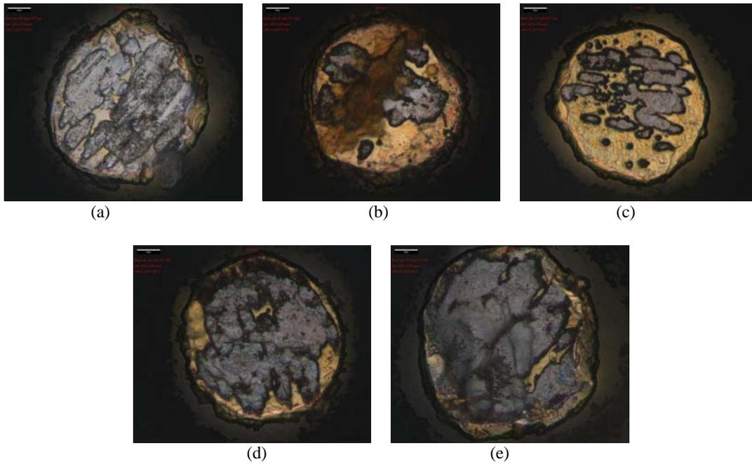
Figure 1. Optical image underside of a typical gold ball after removal from a bondpad for; (a) Run 1 (b) Run 2 (c) Run 3 (d) Run 4 and (e) Run 5.
