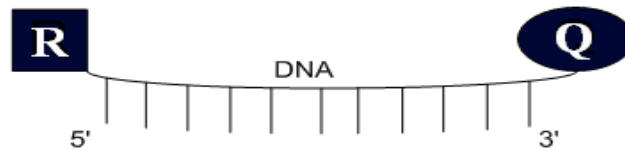
Figure 1: Illustration of the structure of a TaqMan DNA probe. Here, R and Q denote the reporter and quencher fluorophores, respectively
