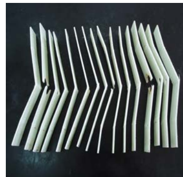
Figure 7: Final form of the damaged shape of the laminated plates
