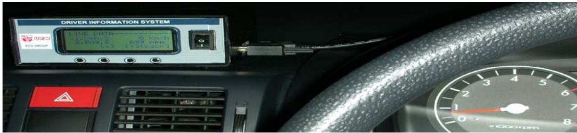
Figure 6: Proposed DIS is interfaced with Hundai Getz car's ECU
