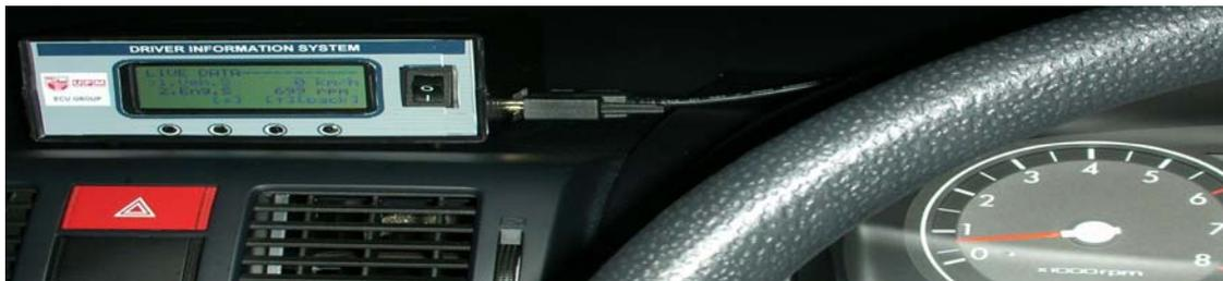
Figure 6: Proposed DIS is interfaced with Hyundai Getz car's ECU
