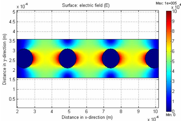
Figure 3: The 2-D representation of the electric field variation in a wire electrode system simulated at 30  $V_{pk-pk}$ . The strongest electric field strength as shown in red can be seen near the electrode edges. As one moves away from the edge of electrodes, the electric field strength becomes weaker.
