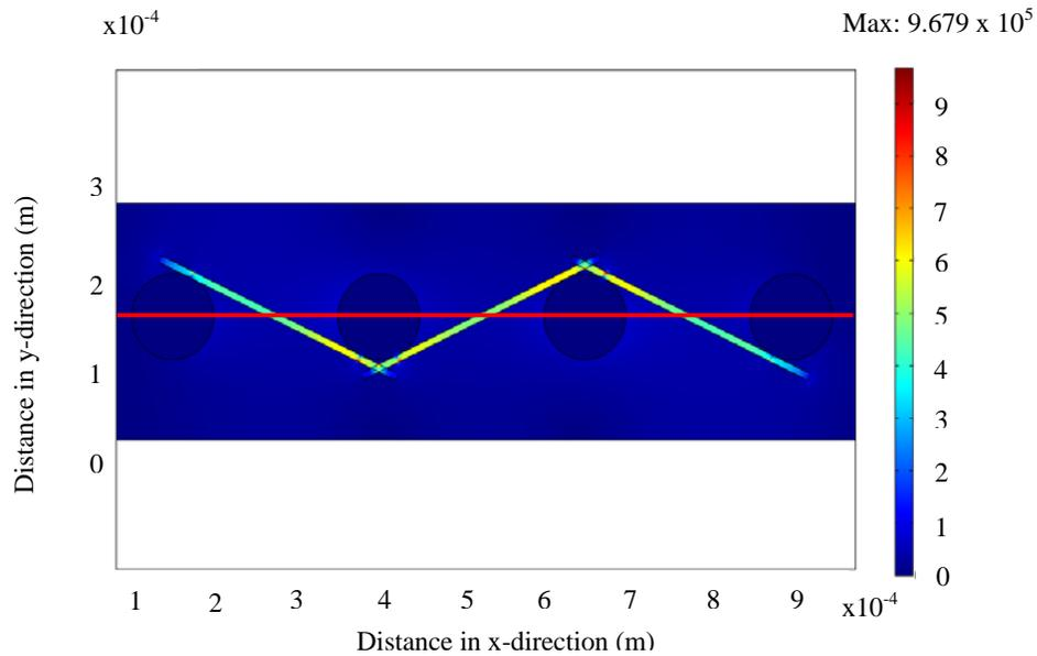
Figure 5: The 2-D electric field surface plot for a wire cloth system with a polyester yarn ( $\epsilon_p = 3.5$ ). The presence of the yarn disturbs the electric field lines and causes a high electric field strength region to be generated at the yarns and reduce the field strength at the vicinity of the yarns.
