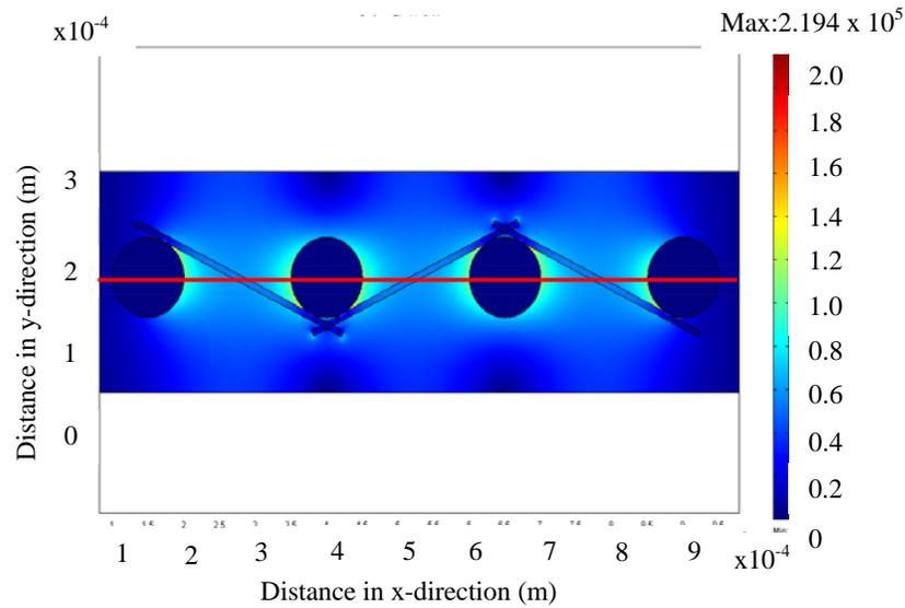
Figure 7: The electric field surface plot for a wire cloth with a yarn having a higher value of electrical permittivity ( $\epsilon_p = 500$ ). The electric fields are disturbed by the high permittivity yarns creating, a high electric field strength region in the surrounding medium instead of inside the yarn as in Figure 3.
