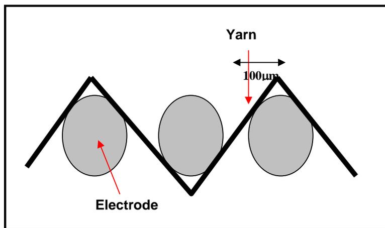
Figure 2: Front view of model wire cloth electrode system used in simulation work
