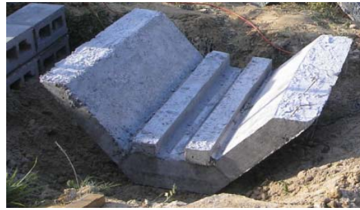
(b) Inverted triangular shell footing.
