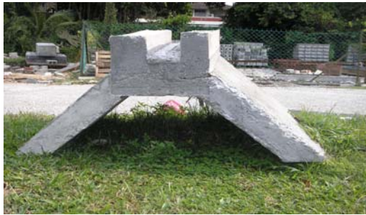
(a) 'Upright' triangular shell footing.
