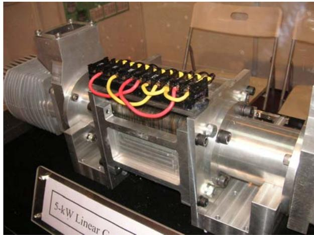
Figure 2: Prototype of linear generator
