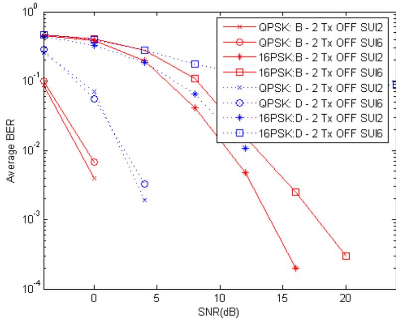
Figure 2: Performance comparison Coded STF-OFDM with 2 Tx OFF employing 30° directional antenna adapting to second-order moment of CIR
