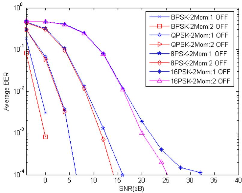
Figure 3: Second-moment-based AdMAS of coded STF-OFDM using directional antenna over SUI6 channels
