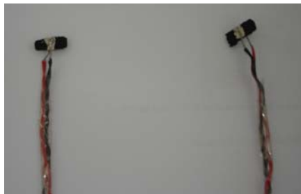
Figure 2: Carbon nanotube pellets with binder
