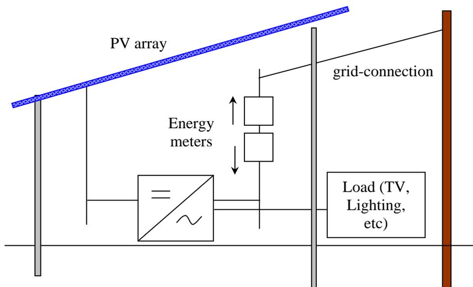
Figure 1: Schematic diagram of the grid-connected PV system.
