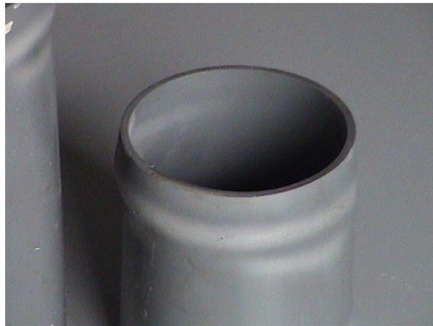
*Figure 11: Shape of failure of pipe specimens without orifice*
