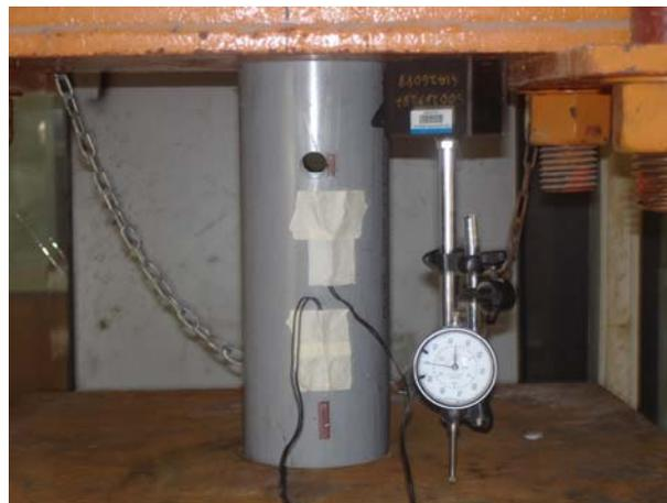
Figure 3: Measuring specimen axial displacements and strains
