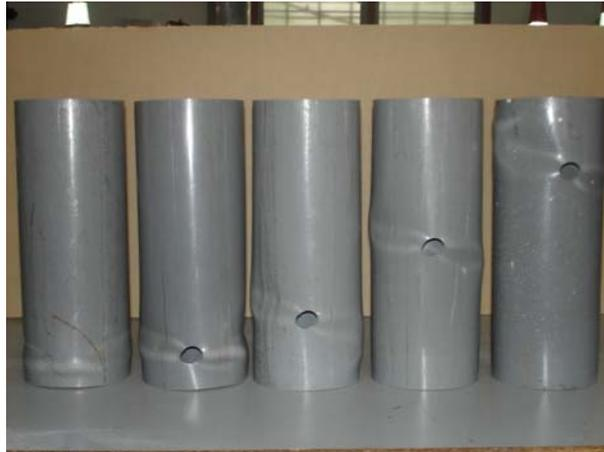
Figure 13: Failure occurred at pipe specimen's orifice
