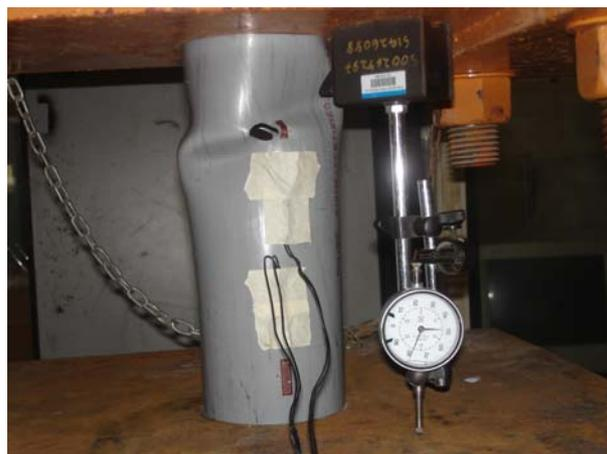
*Figure 12: Failure of pipe specimen during the test*
