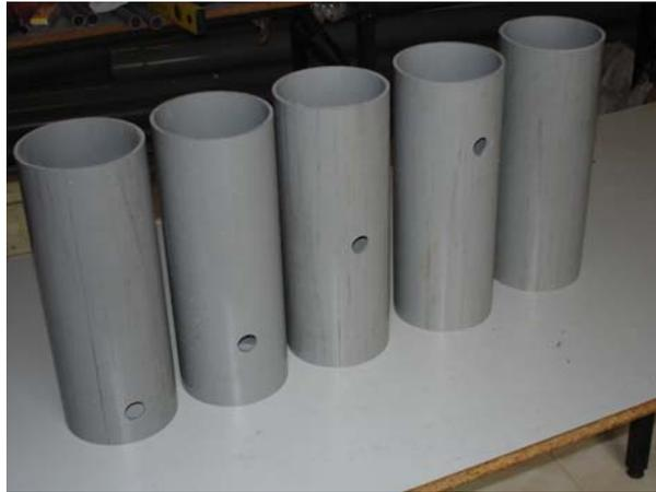
Figure 1: Pipes specimens prepared for test
