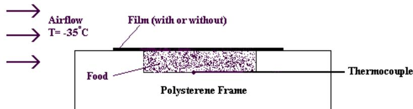
Figure 1: Schematic diagram for an air-blast freezing.
