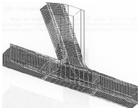
Figure 12: Stress distribution for model AM1
