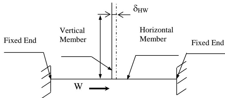
Figure 3: Horizontal member subjected to axial load,  $W$
