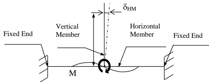
Figure 4: Horizontal member subjected to bending moment
