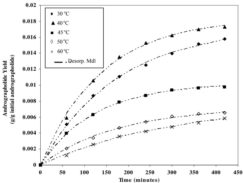
Figure 2: Effect of temperature on extraction yield as a function of time at 10 MPa using 0.375 mm particle size and solvent flow rate of  $3.18 \times 10^{-5}$  kg/s.
