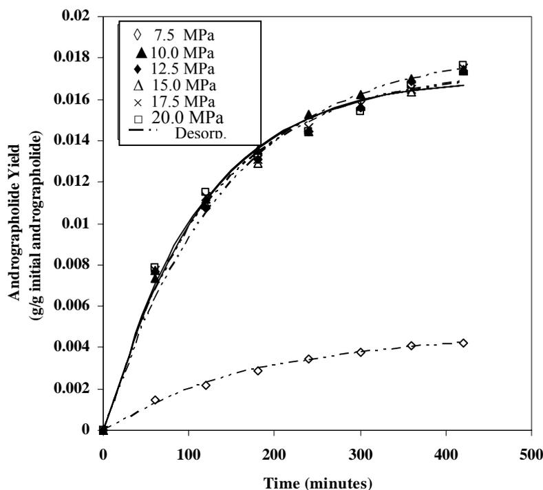
Figure 3: Effect of pressure on extraction yield as a function of time at 40 °C using 0.375 mm particle size and solvent flow rate of  $3.18 \times 10^{-3}$  kg/s.
