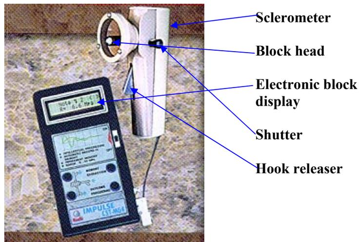
*Figure 1: Concrete Strength Tester, CST-MG4*
