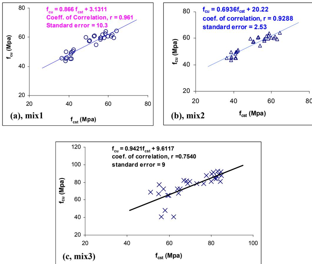
Figure 3: Linear correlation of mean strength by Sclerometric method and cube strength for concrete in series A<sub>12.5</sub> of 12.5mm (max) aggregate size.
