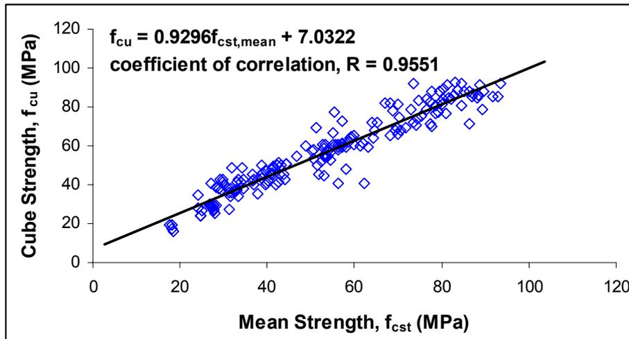
Figure 5: Linear correlation of mean strength by Sclerometric method and cube strength regardless of grade and aggregate size.
