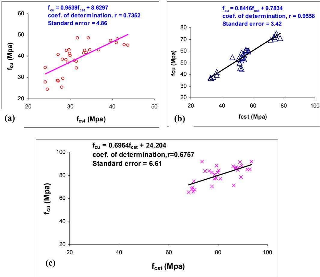
Figure 4: Linear correlation of mean strength by Sclerometric method and cube strength for concrete in series B<sub>20</sub> of 20mm (max) aggregate size.
