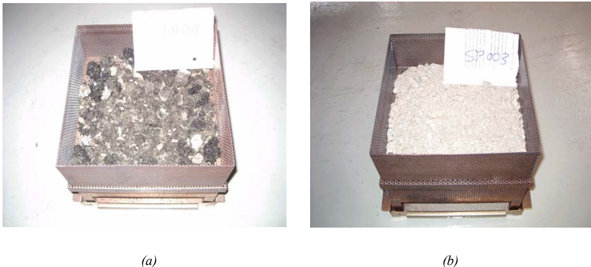
Figure 2: RAP samples (a) before and (b) after extraction process using the ignition oven method
