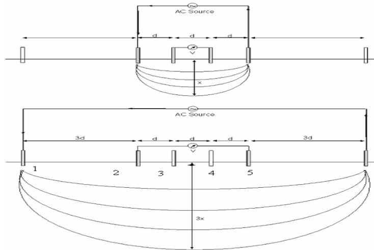
Fig. 2: Schematic of Configuration A-Shallow <30 cm (top) and B-Deep <90 cm(below).
