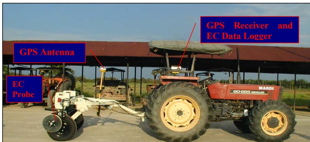
Fig. 3: VerisEC 3100 and GPS Pulled by a Tractor
